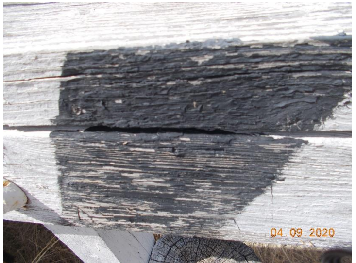
Paint sample M-21-I-LP02. The black paint on wood is considered lead-based paint.
