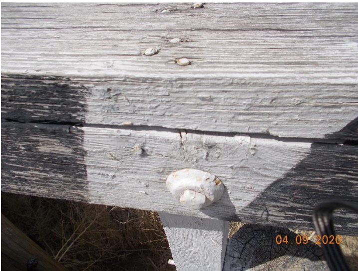
Paint sample M-21-I-LP01. The white paint on wood is considered lead-based paint.
